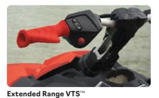
(Variable Trim System) Offers double the range of the regular  $VTS^{\text{\tiny{TM}}}$ for greater ease when executing tricks.
