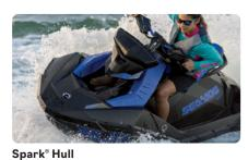
The Spark hull design provides a lightweight and playful platform. The innovative Polytec  $^{\text{TM}}$ material further reduces weight while optimizing performance and efficiency. The color-in molding is more scratch-resistant than fiberglass.
