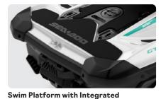
LinQ System Exclusive quick-attach system on a large swim platform that allows for easy installation of accessories.
