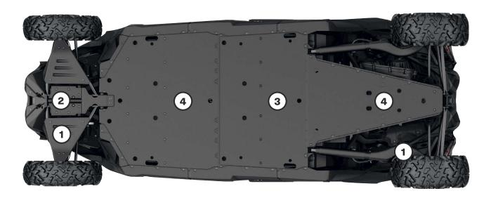
Our Plastic Plates glide smoothly and silently over obstacles, offering great protection in rough terrain. Made of abrasion-resistant thermoformed  $\frac{3}{8}$ " (10 mm) thick High Molecular Weight Polyethylene (HMWPE).
