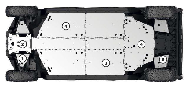
For ultimate durability and strength, all our Aluminum Skid Plates are made with High Strength 5052 H32 Aluminum <sup>3</sup>/<sub>16</sub>" (4.5 mm) thick.
